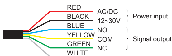
Input and output wiring
